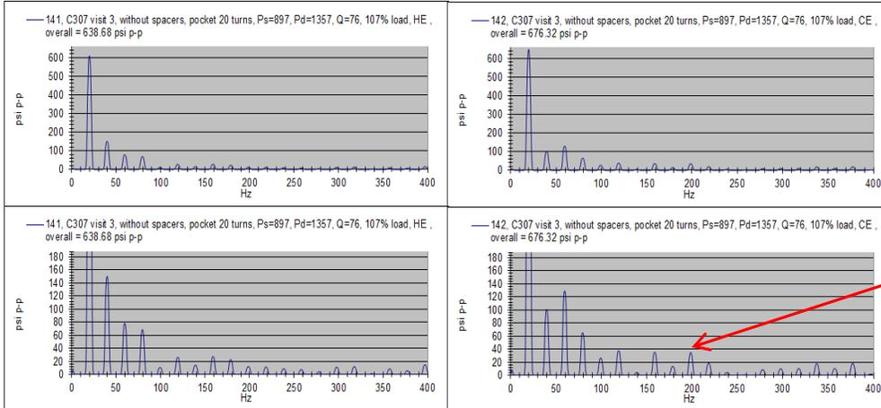
The pressure data here is the spectrum on a 12" cylinder pressure time curve. This cylinder had a very high vibration at 200 Hz. The 30 psi p-p at 200 Hz turns into a force of 3400 pounds exciting the horizontal cylinder MNF.
